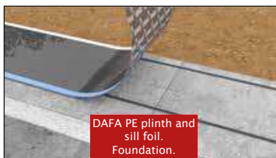
Sealing against plinth / foundation.
