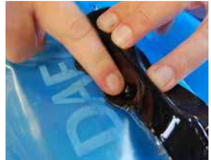
Then flip DMS over the break / item and secure it by pressing it down firmly.
