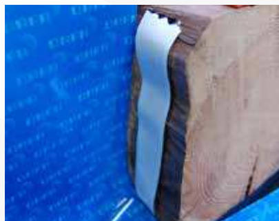
Fix DMS on the beam (remove half of the backing sheet).
