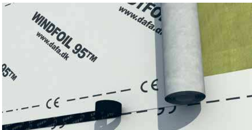
DAFA WindFoil 95 is installed as a wind barrier with a minimum overlap of 150 mm and free joints are taped using DAFA UV tape.
